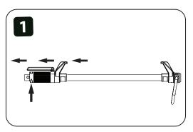
1. Remove all dirt, grit, liquids, greases and oils prior to installation. Press lock button and slide adjustable paw to widest position.
