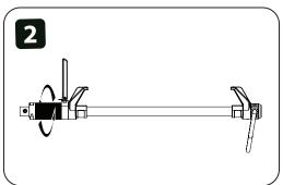
2. Fully loosen nut by turning counterclockwise.
