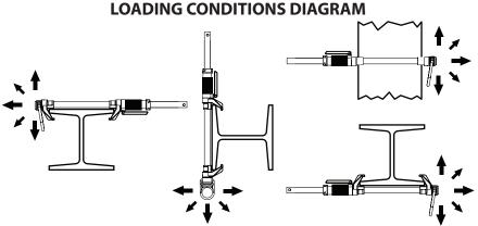
\*Note: Placement at or below a user's working height requires integration of a compatible ANSI Z359.1 shock-absorbing lanyard that does not allow user to extend more than 6 feet (1.8m) (in any direction) from the anchorage connector before shock absorber is activated. Beam anchor must be attached to I-beam flange facing the user (top flange if above, bottom flange if below, etc.).
