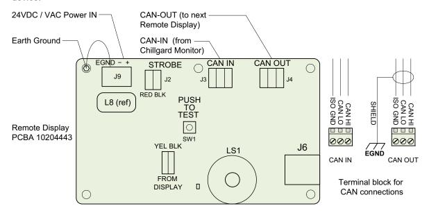
Fig. 12 Remote Display Wiring Diagram
