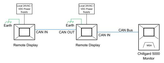
Fig. 9 Two remote displays using "Daisy Chain" configuration. CAN IN of the first remote display must be connected to the Chillgard 5000
