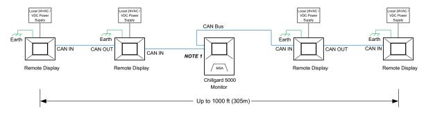
Fig. 10 Connecting four remote displays to a single Chillgard 5000 Monitor
