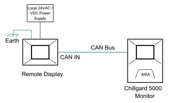
Fig. 7 Single remote display connection
