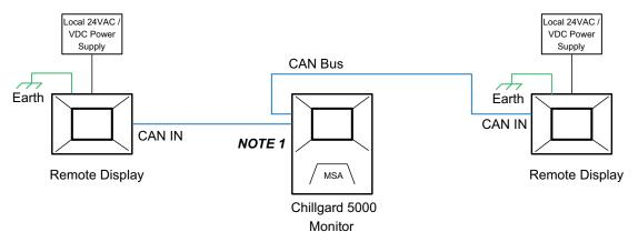
Fig. 8 Two remote displays using separate CAN bus runs
